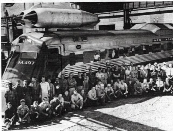
WORLD'S FIRST JET LOCOMOTIVE BUILT AT COLLINGWOOD DIESEL LOCOMOTIVE SHOP-JULY 1966 The M-497 is still America's fastest train and the world's speediest self-propelled locomotive. (Credit: Don Wetzel)
