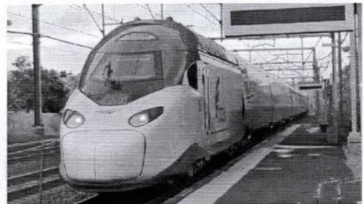
Like the current Acela trains, the new ones have an electric engine at both ends. (Both photos taken at Readville by Adam Gaffin)
