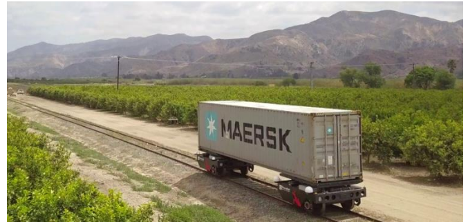
A prototype of the Parallel Systems autonomous container rail system tests in Southern California. Parallel Systems
