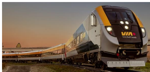
VIA's new corridor equipment will provide bidirectional operation thanks to the first cab cars built for Siemens' Venture equipment.
