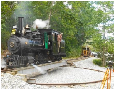
Wiscasset, Waterville & Farmington No. 9, an 1891 Portland Co. 0-4-4, rides the newly installed turntable at Trout Brook Station.
