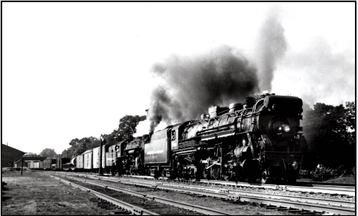
From the archives: B&A double-headed eastbound freight at West Brookfield, Mass. Locos: 2-8-4 #1416 Berkshire-type and 4-6-2 #576 Pacific-type. Stopped for water (tower behind Pacific). Photo by Robert A. Buck 9-7-1947. (Good example of using a freight loco and a passenger loco to power a freight-Ed.)
