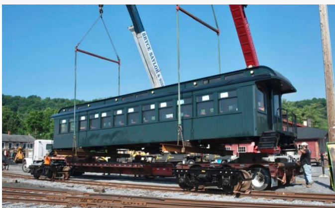
The first of four new East Broad Top passenger cars is lifted off the truck that brought it from its builder in Bellingham, Wash. (Dan Cupper)
