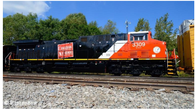
CN 3309, a Wabtec AC44C6M rebuild upgraded to AC traction and 4, 500 hp in 2022 from DC-traction Dash-9 2598 built in 1998, has been assigned to CN’s Executive Train for the past few months.
