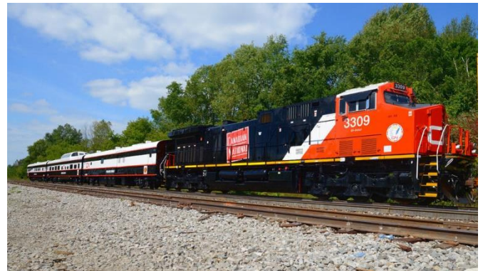
CN 3309, a Wabtec AC44C6M rebuild upgraded to AC traction and 4, 500 hp in 2022 from DC-traction Dash-9 2598 built in 1998, has been assigned to CN’s Executive Train for the past few months.
